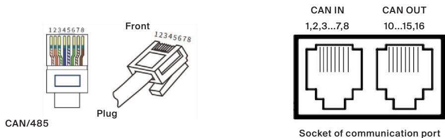
Figure 2-2 CAN/485 Interface Definition
