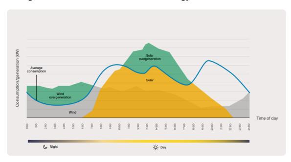
In the Netherlands in particular, with the presence of a net energy metering (NEM; "salderingsregeling" in Dutch) scheme, this is exaggerated, as owners of residential solar systems are incentivized to maximize their energy export to the grid. During sunny hours where overall energy consumption is low, this puts extra pressure on the grid. So, the higher the generation of energy when demand for energy consumption is low, the more difficult the grid management becomes.
