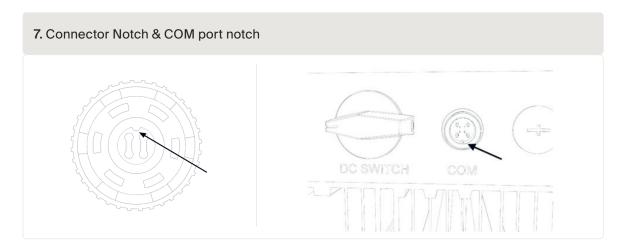
**ATTENTION!** Make sure that the position of the connecting piece of the stick is correct. Place the small notch on the connection point correctly so that the numbering of the 4-pin connector matches the numbering on the inverter.
