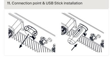
**WARNING!** Keep the 4G stick away from large metal objects and electrical appliances with magnetic fields such as microwave, refrigerator, mobile phone, concrete walls, solar panels and metal walls to ensure the quality of communication.
