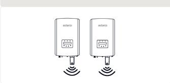
Inverter(s) communicate via 4G STICK D with a public mobile network or via WiFi with local router
