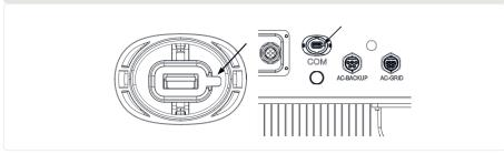
2. Press both sides of the USB port protective cover to open it. Align the 4G data logger with the USB port groove of the inverter and install directly.
