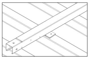
3. Place the beam on the roof with the friction plates on the crowns of the roof plate.
