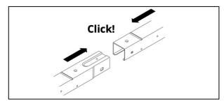
4. Place the base units on the roof according to the installation plan and slide them together as far as the stop.
