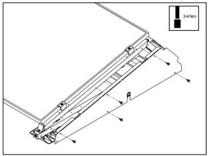
4. Place the side plate on the system. If necessary, press the cables into the cable protector. Screw the side plate with the five screws.
