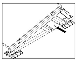
1. When mounting Autarco Matrix, place the ballast plates more inwards or grind them down so that they are flush with the base unit.
