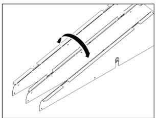
3. Fold over the top edge of the side plate. You can use the side plate for both the left and right sides of the mounting system.
