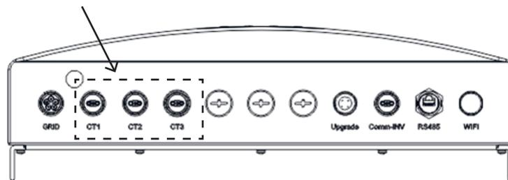
5. Connect RS485 communication cables between inverters and PELD Comm-INV port.
