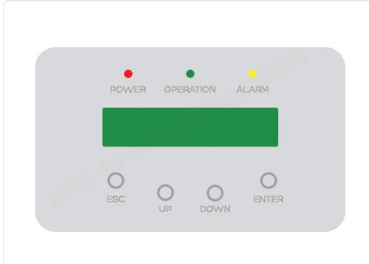
There are four keys at the front panel of the PELD (from left to right): ESC, UP, DOWN and ENTER keys. The keypad is used for:
